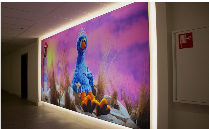
Office, Netherlands. Back-lit wall frame. Dim: 4.60 x 1.80 m. Thickness 140 mm. Translucent print covering
