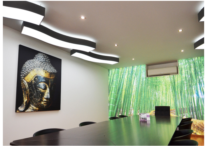
Meeting room, France. Luminous frame (ceiling). Dim: 1.40 m x 0.95 m. Thickness 140 mm. Translucent white covering. Wall frame. Dim. 1.15 m x 1.45 m. Thickness 43 mm. Print covering.
