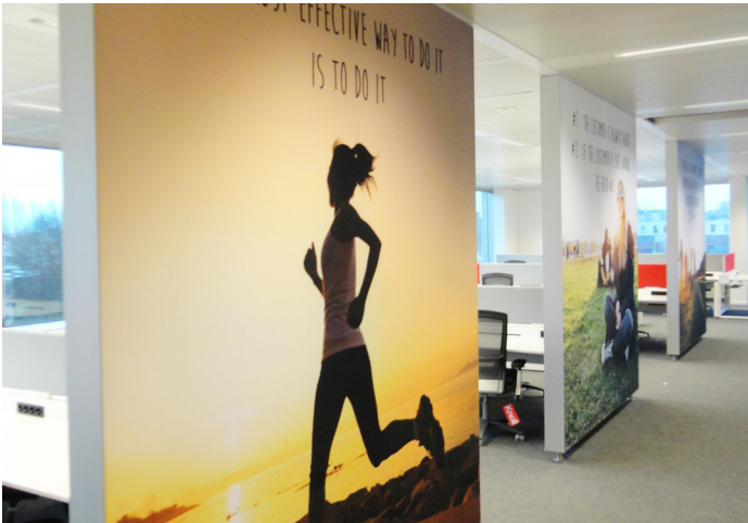
Offices, Belgium. Mobile dividers. Dim: 2.80 m x 2.20 m. Thickness 100 mm. Translucent print covering
