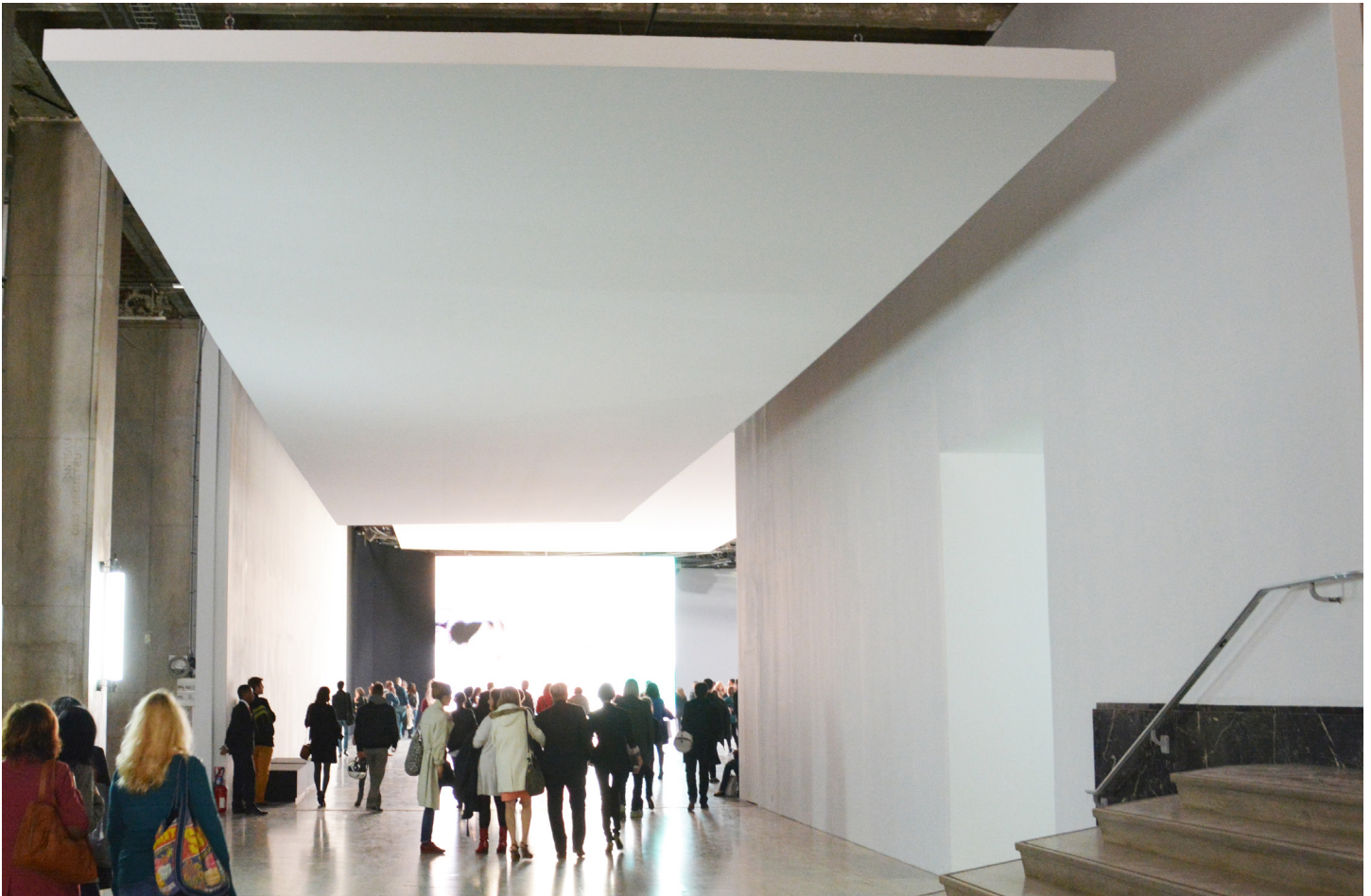
Office, Netherlands. Back-lit wall frame. Dim: 4.60 x 1.80 m. Thickness 140 mm. Translucent print covering
