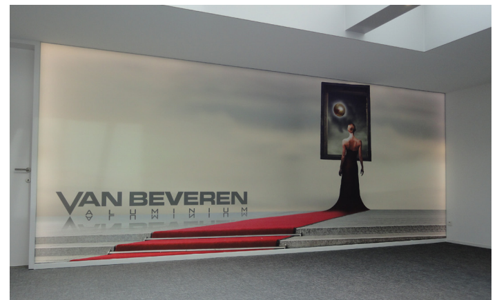
Show-room, Netherlands. Luminous frame. Dim: 4.20 m x 2.00 m. Thickness 140 mm. Translucent print covering
